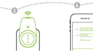
Plug NEO Switch into a power outlet, then press ON/OFF button for 5 seconds and release it. The Wi-Frindicator light will flash quickly. NEO Switch is now ready for synchronization.
